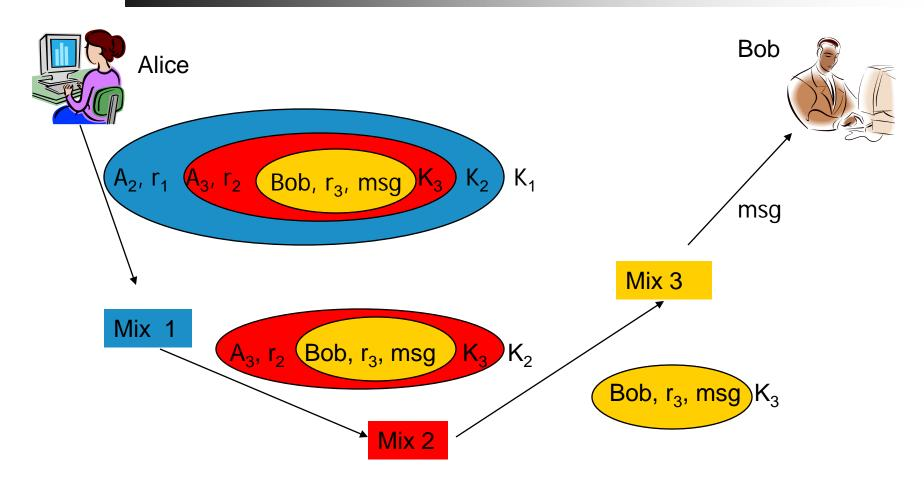
K<sub>i</sub>: public key of Mix<sub>i</sub>, r<sub>i</sub>: random number, A<sub>i</sub>: address of Mix<sub>i</sub>
